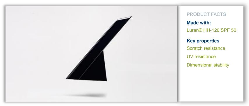
Jaguar Land Rover D-Pillar Cover: Styrolution collaborated with Rosti Mc Kechnie and Jaguar Land Rover to create pillar trims for the Evoque in Luran HH-120 SPF50. Combining high heat stability, excellent uv performance, easy flow, and a lower density compared to PMMA, it provides a cost- effective high-gloss finish without the need to paint.
