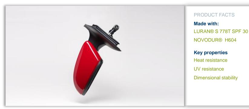
**VW Up mirror:** Volkswagen created the Up mirror housing using Luran S 778T in both the painted and unpainted versions, as it was specifically developed to match the color of the mirror foot made of PA GF. The first application of the superior UV-stable Luran S 778 SPF 30 was used in the mirror base triangle to improve retention of the deep color depth after weathering.
