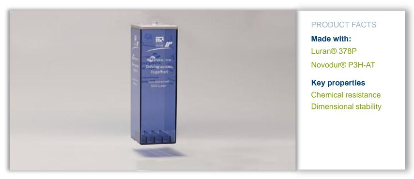
**SERI stationary batteries:** SERI combined two Styrolution materials for the development of its stationary batteries: Luran 378P and Novodur P3H-AT. With both materials offering excellent chemical resistance and high stiffness, Luran was chosen for use in the battery case due to its brilliant transparency, while Novodur P3H-AT was an ideal choice for the top cover given its dimensional stability and strength.
